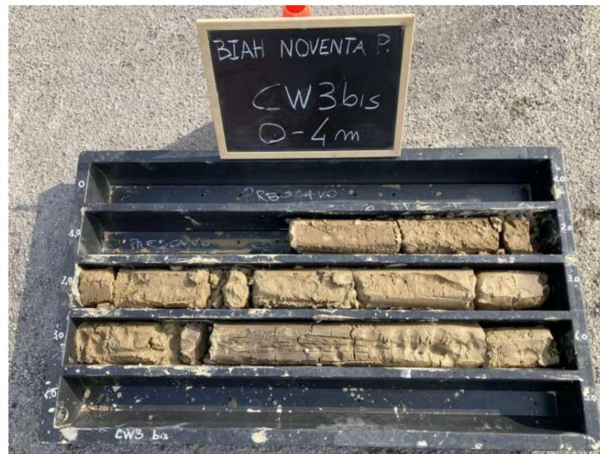
Cassette catalogatrici CW3BIS (4-7 m s.l.m.) / Coring boxes CW3BIS (4-7 m b.g.l.)
