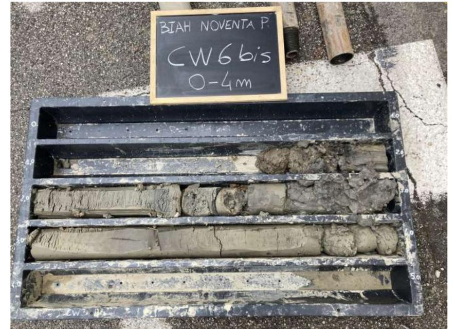
Cassette catalogatrici CW6BIS (4-7 m s.l.m.) / Coring boxes CW6BIS (4-7 m b.g.l.)
