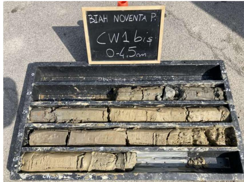
Cassette catalogatrici CW1BIS (4-7 m s.l.m.) / Coring boxes CW1BIS (4-7 m b.g.l.)
